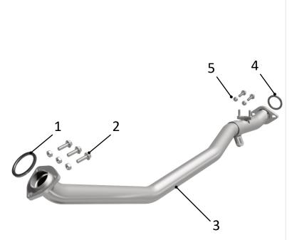
(Carefully read all instructions before installation) Disconnect the vehicle's battery before removal of the OEM exhaust system. This will prevent electrical accidents and will reset the computer if it applies to the vehicle. Remove existing front pipe from the vehicle. Only remove parts that will be replaced. Clean existing flange with a wire brush to ensure proper sealing.
